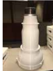
F108 fan shaft with and without 3D printed masking for thermal spray of dia "U"
