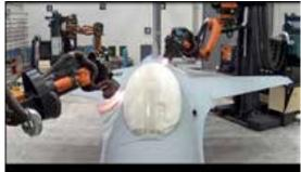
Full Aircraft Robotic Depaint Safe and effective stripping of an entire aircraft
