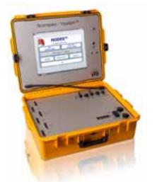
The Ncompass-Voyager<sup>™</sup> man portable Intermittent Fault Detector<sup>™</sup> utilized for EWIS testing on the UH-60, CH-47, C-130, Eurofighter Typhoon, Tornado GR4, Trains, automobiles and consumer electronics.
