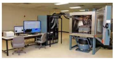
8000 test point Intermittent Fault Detection & Isolation System™ (IFDIS™) testing an F-16 AN/APG-68 Radar System Programmable Signal Processor (PSP)
