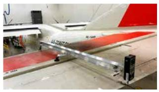
Figure 1: Portable "on-wing" prototype balance tool
