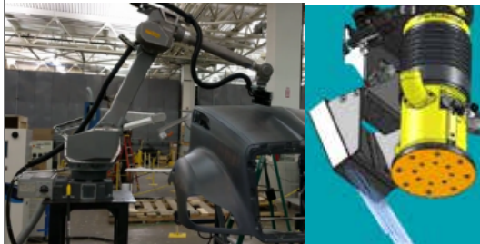
Robot finishing of truck bodies and tool detail
